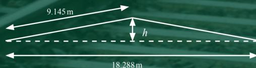
Welded rails are now more common. Welded tracks give a smoother ride, especially at higher speeds, but are more susceptible to buckling as there aren't any gaps. To avoid buckling rails are heated before laying them.
